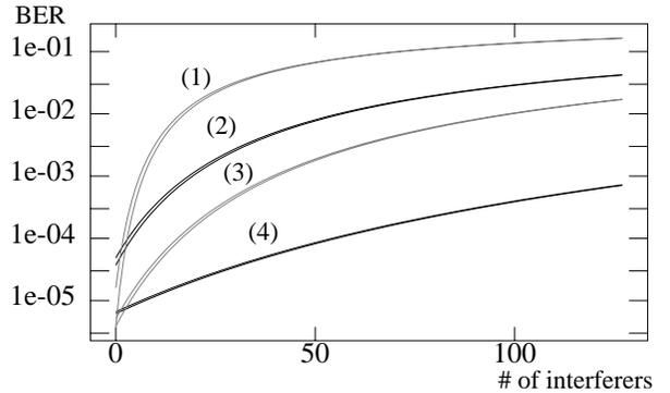
Fig. 3 BER vs. the # of interferers for different Rician  $K$ -factors using MRC:  $K=0$  (1) and  $K=10$  (3) and EGC:  $K=0$  (2) and  $K=10$  (4). Curves are shown for both CLT and LLN approximations. The SNR is 10 dB and  $N = 128$ .
