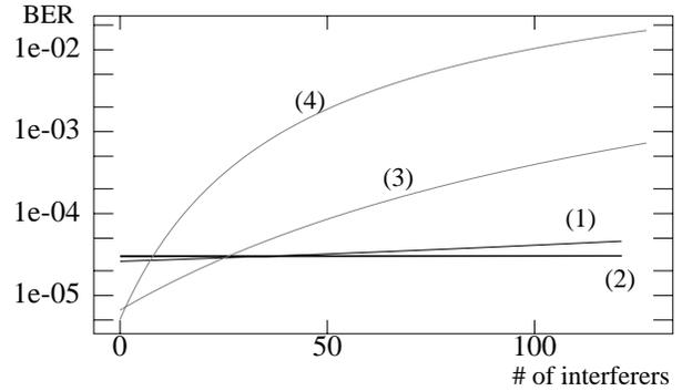
Fig. 5 BER for CE vs. the # of interferers with  $K=10$  for  $\rho_{\text{thresh}}=0.008$  (2) and  $\rho_{\text{thresh}}=0.016$  (1). The SNR is 10 dB,  $p=0.1$ , and  $N=128$ . Plots for EGC (3) and MRC (4) are included for comparison.
