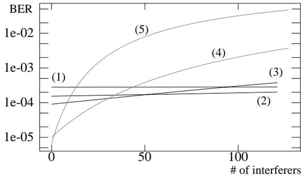
Fig. 4 BER for CE vs. the # of interferers with  $K=5$  for  $\rho_{\text{thresh}}=0.002$  (1),  $\rho_{\text{thresh}}=0.008$  (2), and  $\rho_{\text{thresh}}=0.014$  (3). The SNR is 10 dB,  $p=0.1$ , and  $N=128$ . Plots for EGC (4) and MRC (5) are included for comparison.
