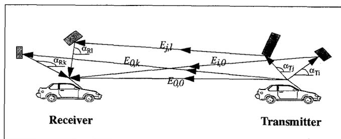
Fig. 1. Mobile-to-mobile propagation channel with scatterers near both antennas.
