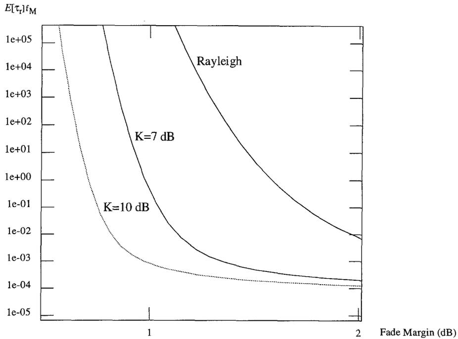
Fig. 4. Average fade duration vs. fade margin for various  $K$ -factors. Equal transmitter and receiver velocities. Equal Rician  $K$ -factors  $K_R$  and  $K_T$ . Maximum Doppler shift for both antennas,  $f_M$ .
