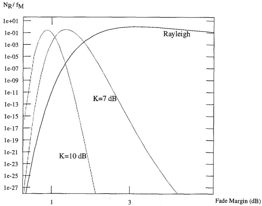
Fig. 3. Normalized level crossing rate vs. fade margin for various Rician  $K$ -factors. Equal transmitter and receiver velocities. Equal Rician  $K$ -factors  $K_R$  and  $K_T$ . Maximum Doppler shift for both antennas,  $f_M$ .  $K = -30$  dB approximates Rayleigh fading.
