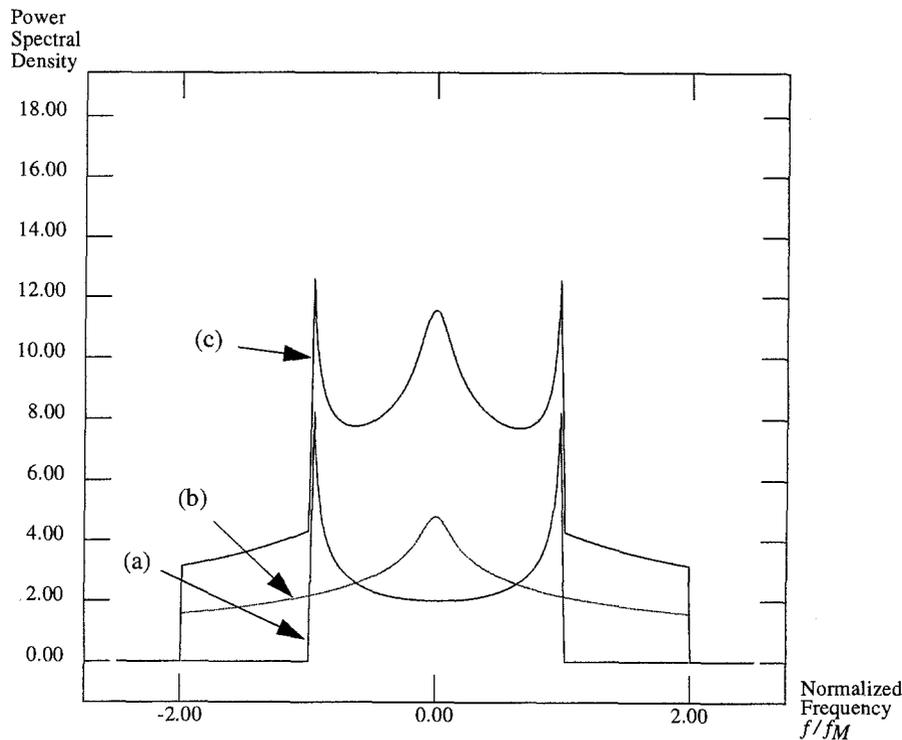
Fig. 2. RF spectra of mobile-to-mobile radio channel with equal transmitter and receiver velocities. (a) Reflections solely at either receiver or transmitter. (b) Reflections at both receiver and transmitter. (c) Summation of (a) and (b).
