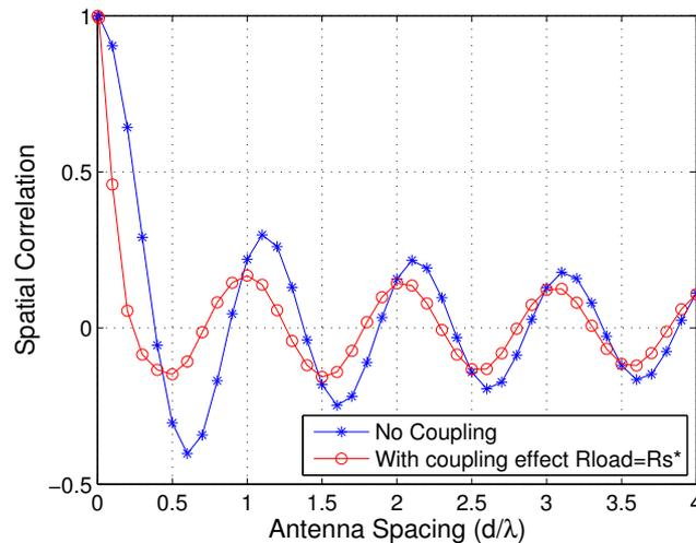
Figure 2: Effective spatial correlation due to coupling for two side-by-side  $\lambda/2$  dipole antennas with  $Z_{\text{load}} = Z_s^*$ .
