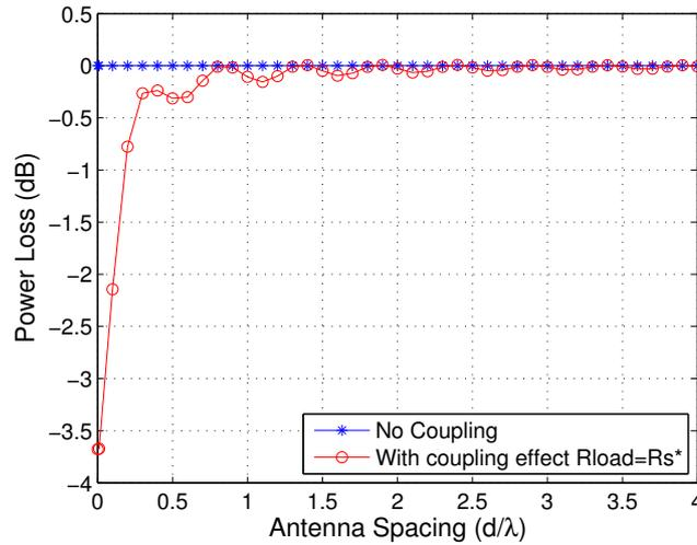
Figure 1: Power loss due to coupling for two side-by-side  $\lambda/2$  dipole antennas with  $Z_{\text{load}} = Z_s^*$ .
