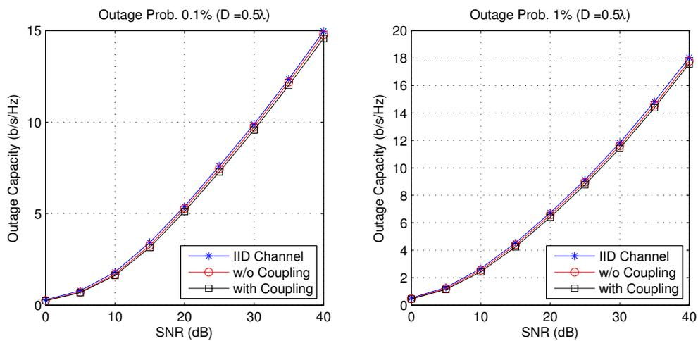
Figure 5: Outage capacity as a function of the SNR ( $D=0.5$ ) .
