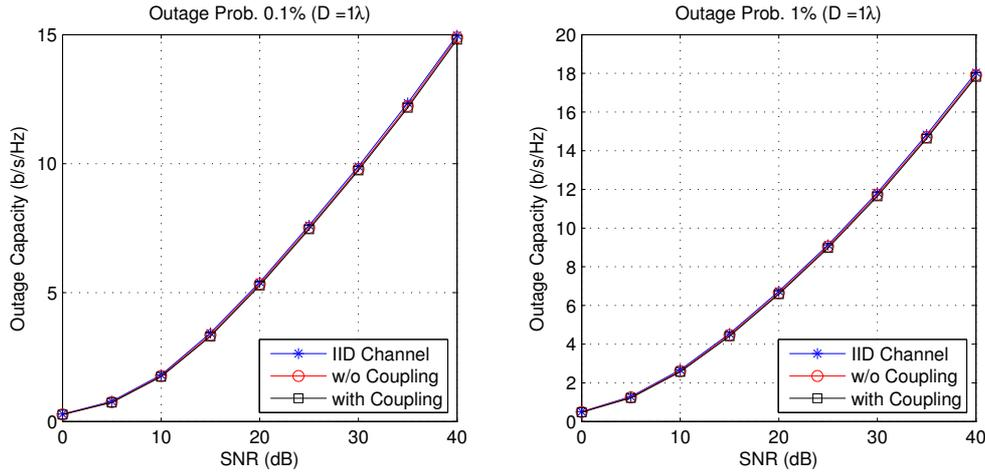
Figure 6: Outage capacity as a function of the SNR ( $D=1$ ) .
