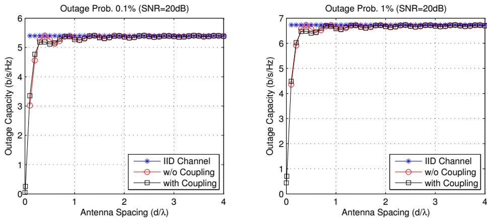
Figure 4: Outage capacity as a function of the antenna spacing (SNR=20dB) .
