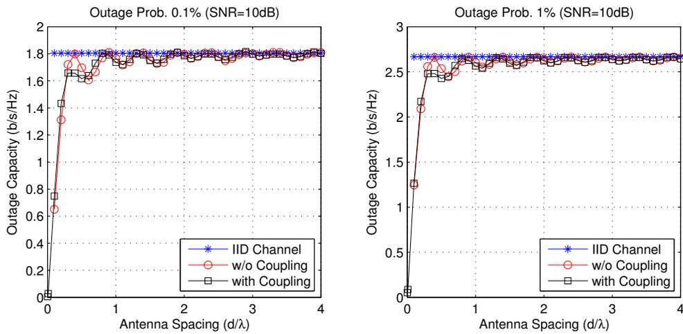
Figure 3: Outage capacity as a function of the antenna spacing (SNR=10dB) .
