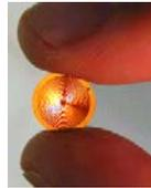
Implant blood pressure flow sensor (CardioMEMS)
